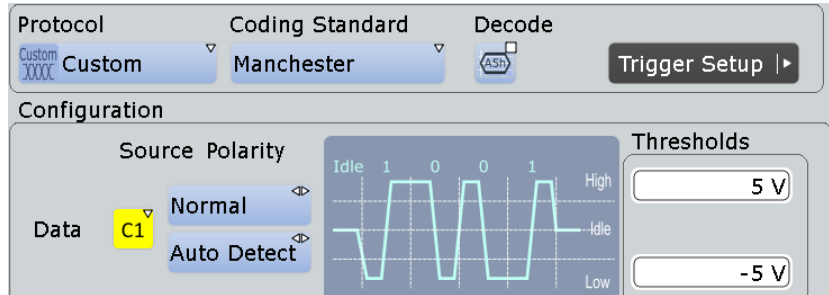
Figure 13-81: Custom serial bus coding configuration Manchester
