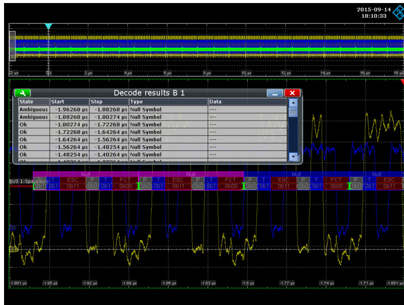
Figure 13-115: Decoded SpaceWire signal with ambiguous bits
